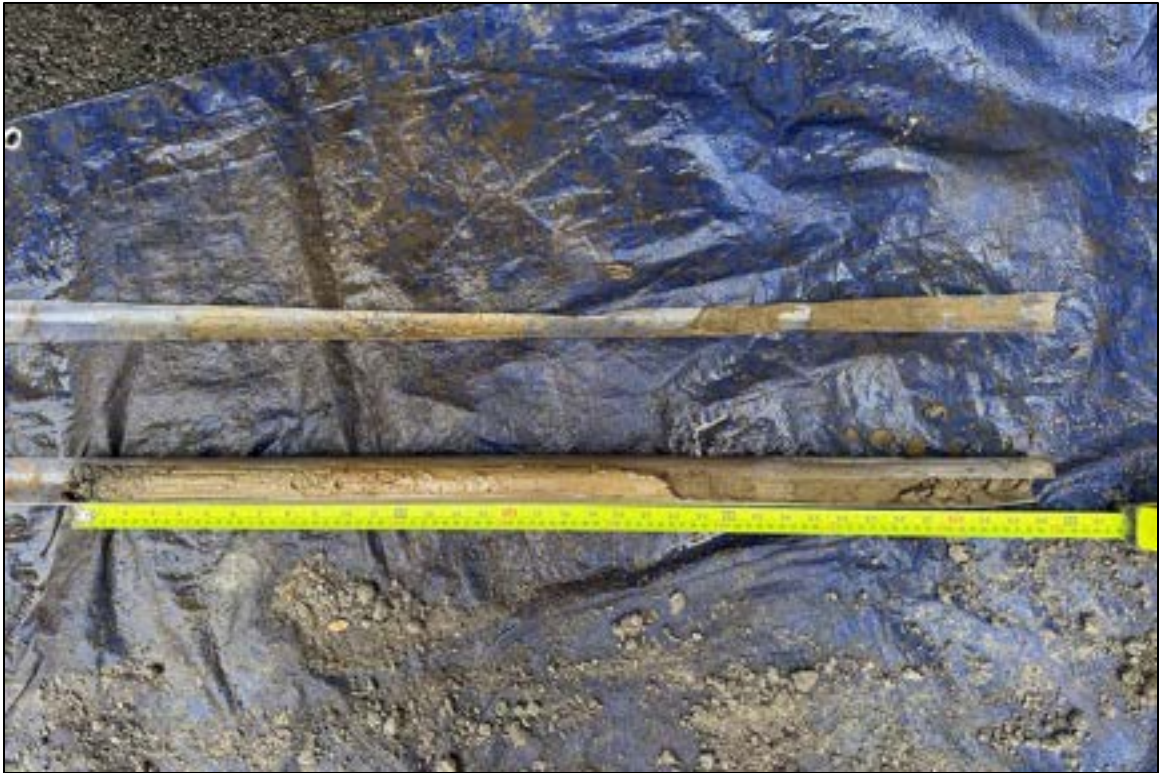
Figure 14. Third core sample from GP-1 showing transition from fill to post glacial sediments between 8 and 11 fbs, depth increases left to right.
